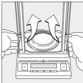
Removing and Cleaning the Weighing Pan:
