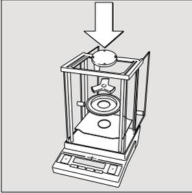
Balances/Scales with an Analytical Draft Shield Chamber:
